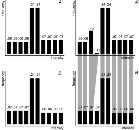
Figure 1: Incorrect histogram specification. *A*) Original histogram. *B*) Specified histogram. *A'*) Resulting histogram using SML histogram specification as in [8]. Using GML also gives erroneous results for this case.
