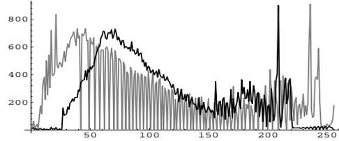
Figure 4: Intensity histograms for the stereo pair. The left and right histograms are respectively in gray and black.
