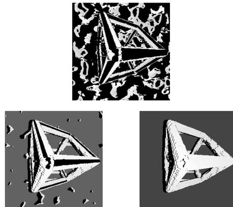
Figure 6: Disparity maps: (Top) with no correction, (Left) with a linear correction model and (Right) with DHW
